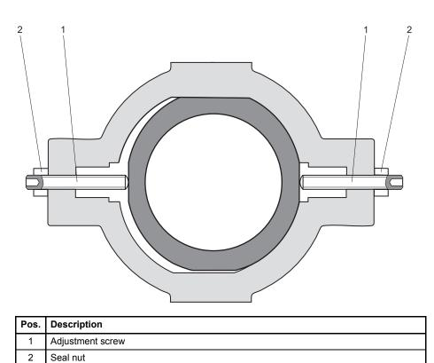
Fig. 10: Mechanical stroke adjustment, B1
