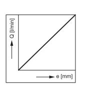
Mechanical Stroke Adjustment, B1
