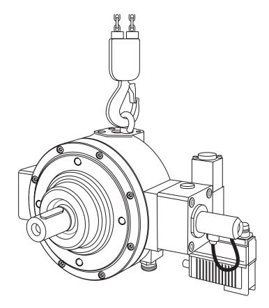
Fig. 17: Transporting Pump with Lifting Tackle
