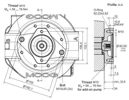
Fig. 22: Adapter flange SAE-A with 9-tooth shaft
