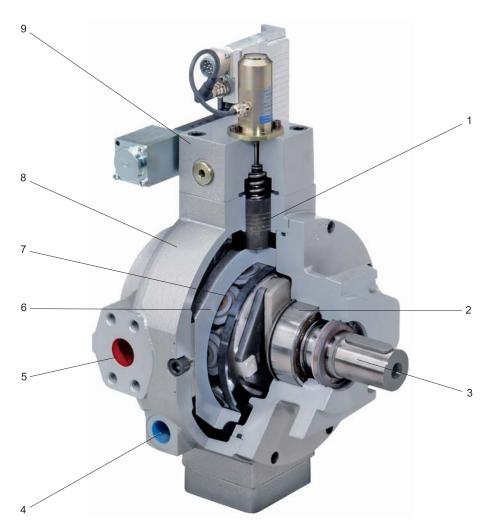
Pos. Description Control piston 1 2 Rolling bearing 3 Drive shaft 4 Drain Port 5 SAE piping connection 6 Sliding stroke ring 7 Slipper pad with working piston Housing 8 9 Compensator
