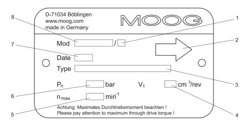
Pos. Marking Additional Information 1 Revision status Rotation direction 2 3 ⇒ Catalog Radial Piston Pump RKP-II Type key 4 displacement 5 Maximum revolutions for low noise operation 6 Maximum operating pressure 7 Date of manufacture in the format MM/YY Model number 8
