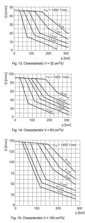
Approximation to the power hyperbola by means of two springs. Referenced on n = 1450 1/min.
