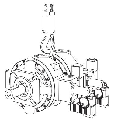
Fig. 18: Transporting Multiple Pumps with Lifting Tackle
